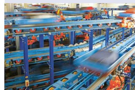
Countless rollers, belts, and motors move the luggage trays with the suitcases from A to B. In addition to the use of more energy-efficient drives, the duration and friction losses in particular will be reduced in order to conserve energy. These measures also increase the intervals at which the system needs to be serviced due to less wear. Performance measurements show an expected saving of approximately 30% by implementing these measures, which corresponds to approximately 7 GWh per year.
