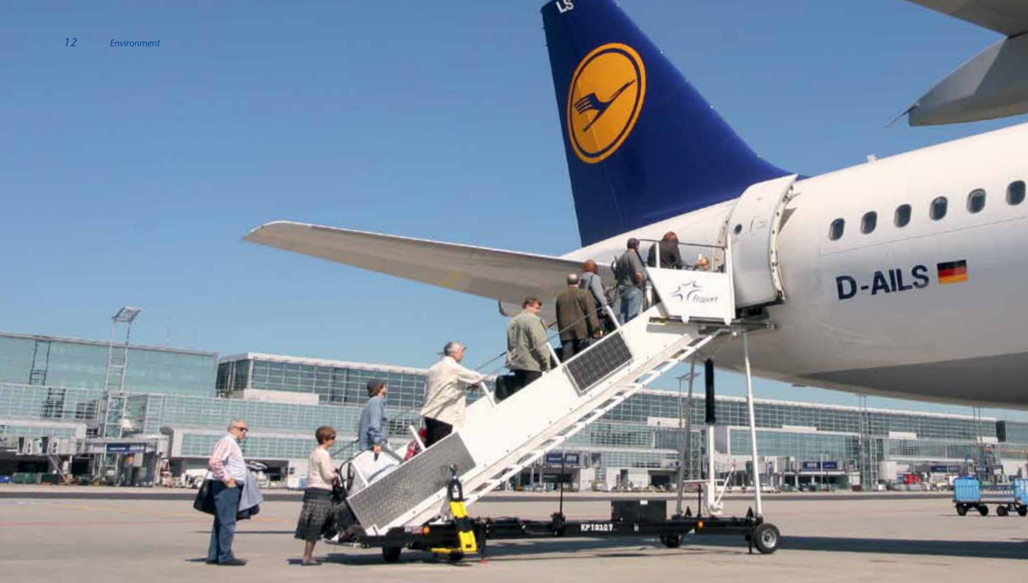
Solar cells generate the energy for the LED illumination used on a large number of passenger escalators at Frankfurt Airport.
