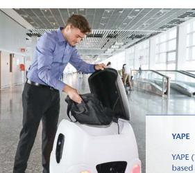
YAPE (Your Autonomous Pony Express), the transport and delivery robot based on artificial intelligence (AI) and equipped with a high-resolution HD map, cameras, and sensors, was deployed in the transit area of the airport during a five-day test phase in September 2019. In addition to studying how it was received by passengers, the requirements for airport infrastructure were also tested by the use of robotics and AI.
