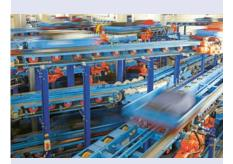
Countless rollers, belts, and motors move the luggage trays with the suitcases from A to B. In addition to the use of more energy-efficient drives, the duration and friction losses in particular will be reduced in order to conserve energy. These measures also increase the intervals at which the system needs to be serviced due to less wear. Performance measurements show an expected saving of approximately 30% by implementing these measures, which corresponds to approximately 7 GWh per year.
